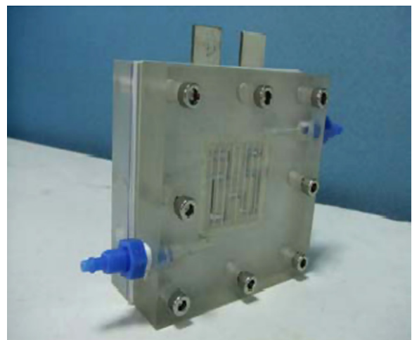
Fig. 8. The assembly of the single cell DMFC test fixture.
